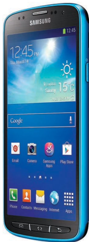
FIG. 2. The Samsung Galaxy S4 is one of several Android phones with high-quality pressure sensors. (Source: www.imgreview.info/samsung-galaxy-s4-active-orange/ )
