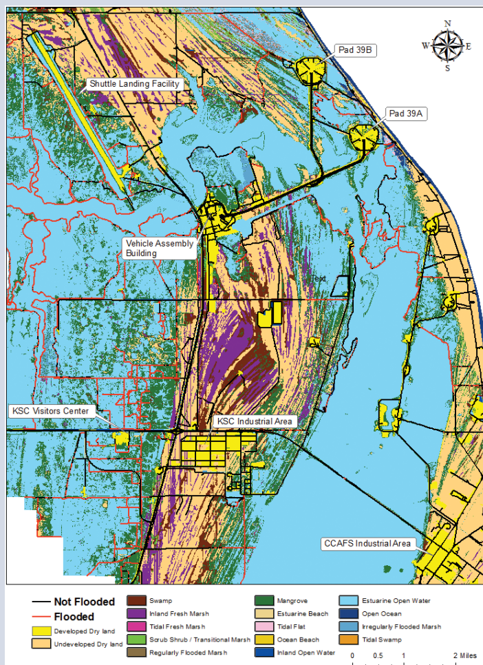
FIG. SBI. Potential flooding in the KSC environs based on the Sea Level Affecting Marshes Model (SLAMM) under a 1.2-m (NAV88) sea level rise scenario. SLAMM output was developed in conjunction with the EPA Indian River Lagoon National Estuaries Program and Industrial Economics, Inc. (2011) utilizing CASI-developed climate change scenarios for KSC. In this scenario, most current wetlands in the region convert to open water and mangrove forest. Road inundation, during the annual fall period of maximum monthly mean sea levels, includes 11.5%, 30.5%, and 60% of primary (main arteries), secondary (paved), and tertiary (unpaved) roads, respectively. These roads are at or below 1.2-m elevation, so any combination of sea level rise, storm surge, wave-induced runup, and wind-driven seiches (standing waves) that raise the lagoon level to 1.2 m will inundate these areas. Duration of inundation will depend on magnitude and duration of individual events. These event-based inundations are projected to increase in frequency and magnitude as sea level rises from current elevation.
